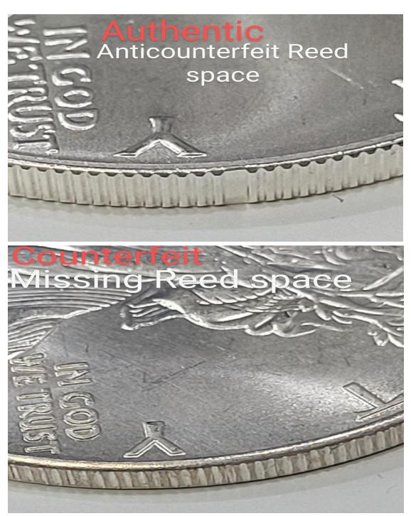
These coins are also too small in diameter, at approximately 39.94mm, measured with a digital caliper, compared to the U.S. Mint originals at 40.6mm. The counterfeit example also measures approximately 2.61mm thick, while the authentic U.S. example measures approximately 2.87mm thick, measured at the same time instore with the same digital caliper.
